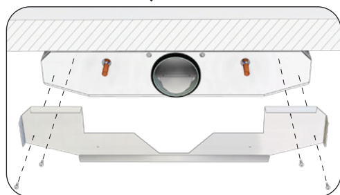
Self drilling screws for bracket on gable of beam. Screws (x4) included.
