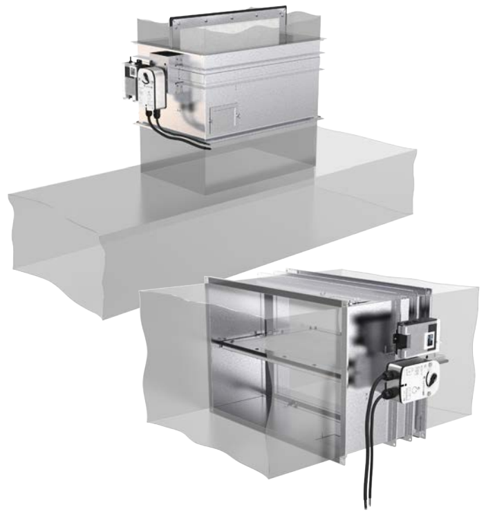
Fig. 2: Installatin of the rectangular smoke damper DKIS1 onto and into the duct running through the vertical supporting construction ( v_{ed} - see the fire resistivity on the page 3)
